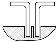
TYPICAL CANE STYLE BOLT DETAIL
