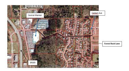
Forest Rock Lane, an important neighborhood collector in our City Network, was built 20 years ago and is in need of an upgrade. Steepness of the road, subsurface water flow, road base and asphalt thickness have all been contributing factors to condition of the road. This project will rebuild the road base, install trench drains, and thicker asphalt to improve the road. The road will be upgraded from the Central Market
