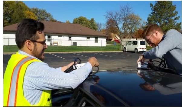
Attaching LPR cameras to a car roof with magnets.
