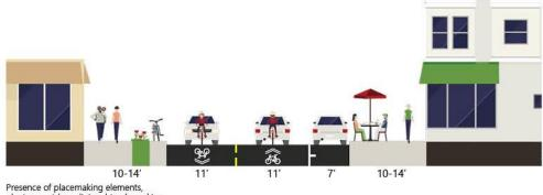
Figure 3. Main Street Cross Section
