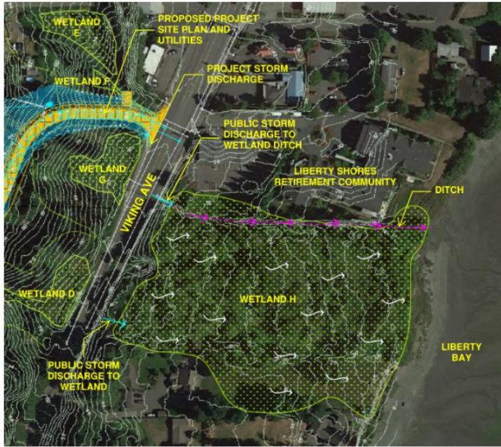
Figure 6-6: Stormwater Ditch Through Offsite Wetland H
