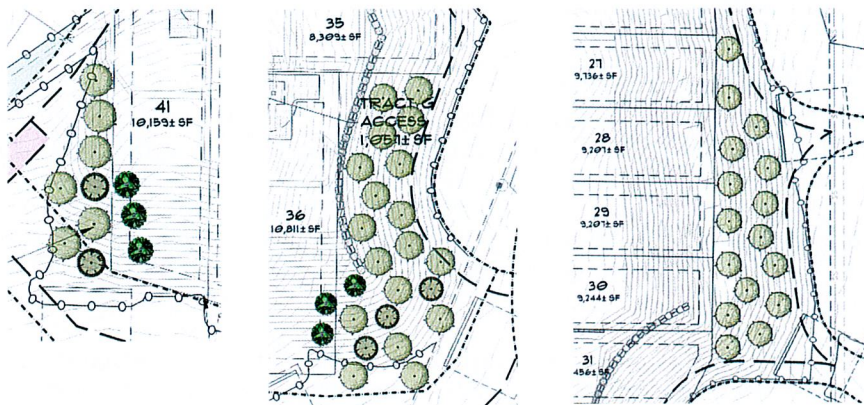
Tree retention planting on areas of reinforced soil slope.
