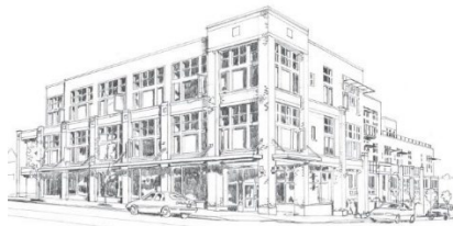
Conceptual design of a mixed-use building with retail commercial on the first floor, office on the second floor, and residences on the third floor. Design elements include facade modulation, roofline cascade, rooftop deck, awnings, varied facade materials, recessed and frame windows and ornamental pilasters.
